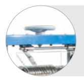
BLADE ELEVATION FEATURE ADJUSTABLE TO CABLE SIZE
